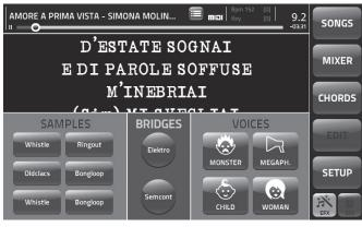
On the left of the page there are 6 touch pads associated with 6 different sampled effects (Samples). The Merish 3 memory contains 60 Samples.
