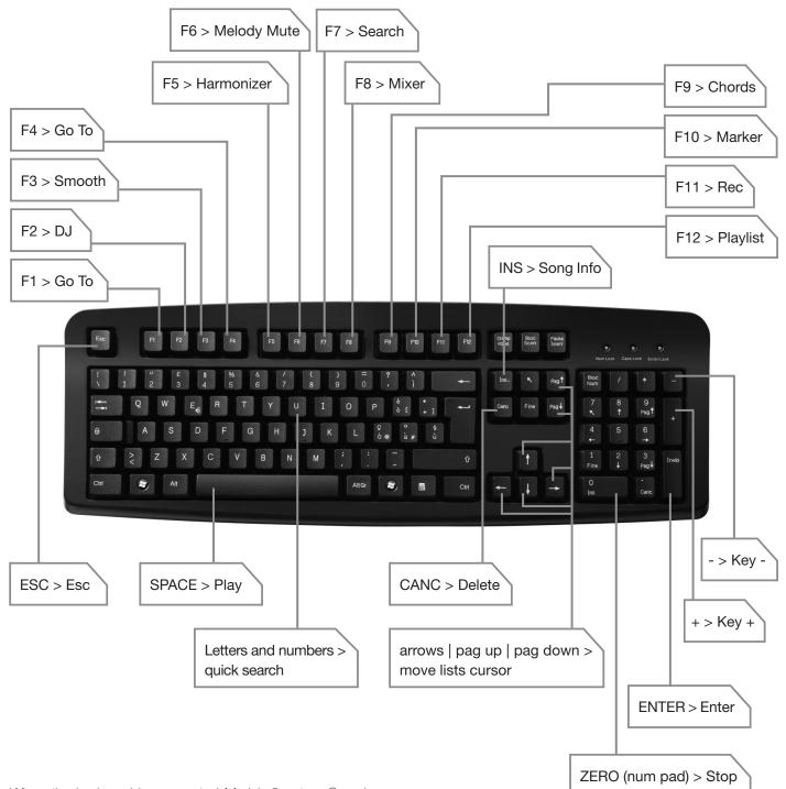
When the keyboard is connected Merish 3 enters Search mode as soon as it reads the typed text string; for example, if you write "Love" the text string will appear at the bottom of the page. Now press "Enter" and Merish 3 will perform a search based on the string. This means there's no need to press "Search" or "Songs" to browse the songs.
