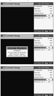
N.B. when the Merish2 is switched on, the Phantom power supplies are always off.
