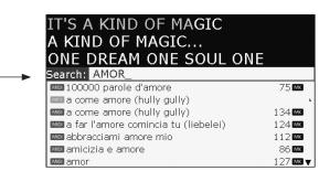
Searching is easy even without the PC keyboard. Press A/Z Search to display the alphabet on screen. Type text by moving the cursor with the Alpha Dial and confirming every letter with the illuminating Enter button. Press the A/Z Search button to confirm the search.
