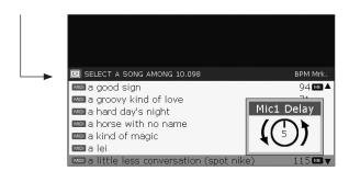
The arrow around the circle (which represents the knob) tells us that to modify the value we need to turn the knob to the left, to the setting that coincides with the current value. Upon reaching the position that corresponds to the value saved (5), we can increase or decrease the setting.
