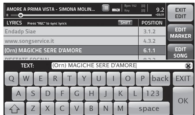
To move the sync point simply touch the Position Box associated with the line of lyrics you want to move and then turn the Alpha Dial.
