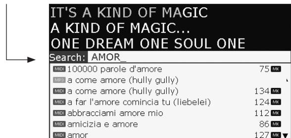
Searching is easy even without the PC keyboard. Press A/Z Search to display the alphabet on screen. Type text by moving the cursor with the Alpha Dial and confirming every letter with the illuminating Enter button. Press the A/Z Search button to confirm the search.
